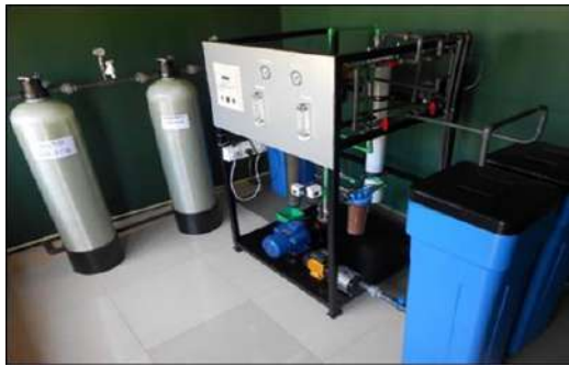
Figure 2. The Brackish Water Reverse Osmosis Plant with a capacity of 10 tons/ day was developed by Sri Lanka Navy.
