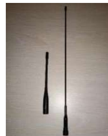
Figure 4. Two types of whip Antennas
