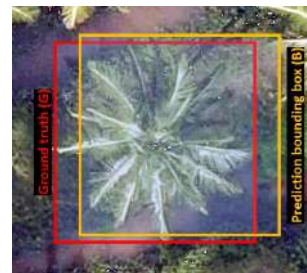
Figure 8. Intersection over the union of ground truth and prediction bounding box.
